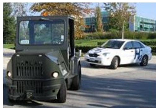
Figure 8: Fuel cell powered Harlan tugger
