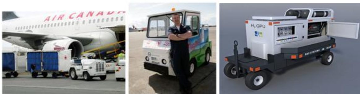
Figure 7: Fuel cell powered ground support equipment prototype units
