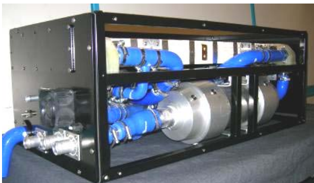
Figure 14: Prototype APU incorporating Ballard fuel cells
