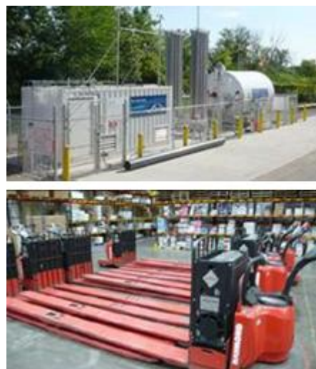
Figure 6: Fuel cell forklifts and hydrogen fuelling station at Sysco
