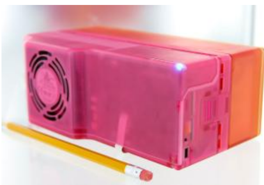
Figure 13: Prototype PEM fuel cell micro-generator (45W net, 250Wh energy storage)
