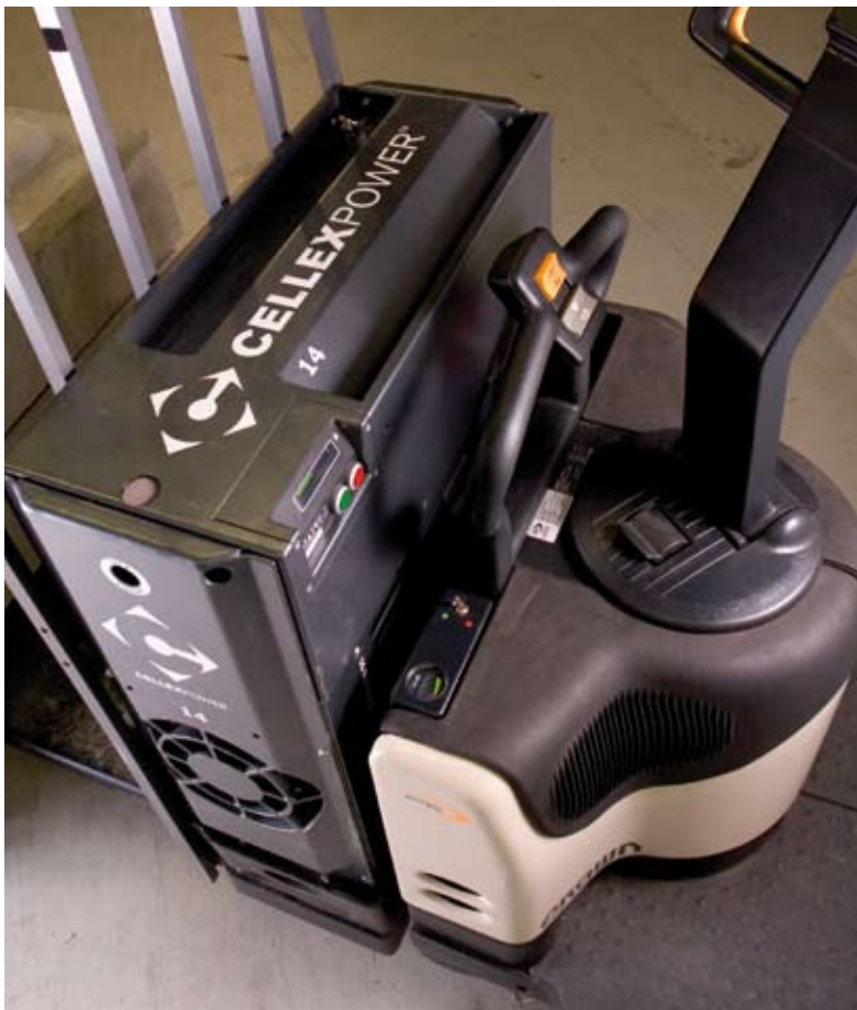
Packaged to transparently replace industrial batteries for easy customer adoption
