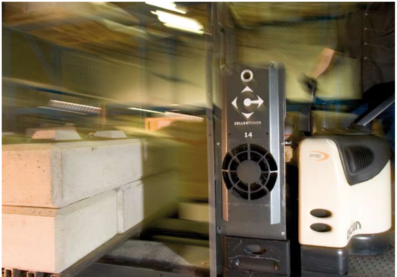
A CX-P150 power unit on board a Class 3 rider pallet truck used in in customer field trials
