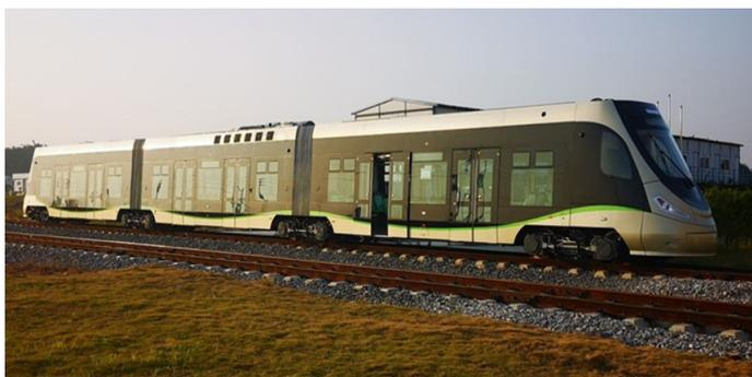
The fuel cell tram has currently recorded a total of more than 425,000km driven during 35,000 operating hours, while meeting the target of 97% fuel cell availability.
